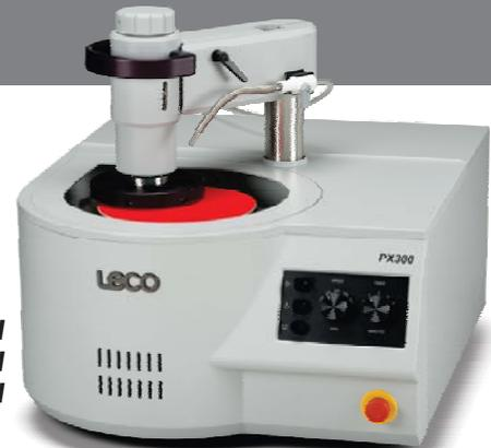
LECO's PX300 Grinder/Polisher Series emphasizes ease-of-use while delivering specimens that are ideal for microhardness or microstructural evaluation. Our PX300 provides an efficient, safe, reliable, and clean grinding/polishing solution for low-volume laboratories.
