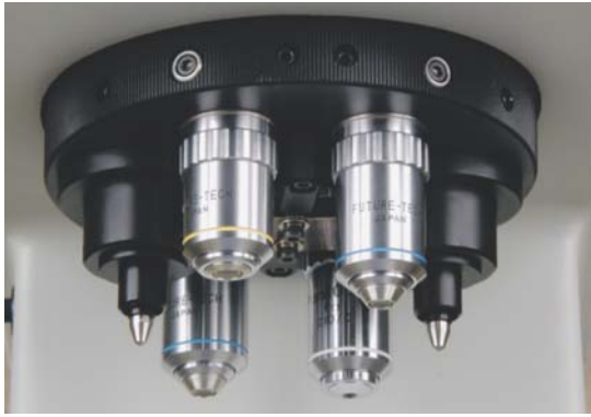
Automatic Turret (AT) and manual turret, with up to 2 indenters and 4 objective positions
