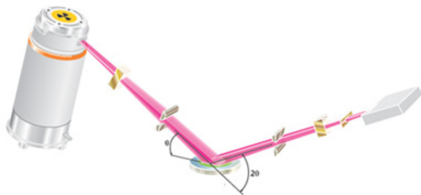
Schematic representation of a X-ray diffractometer for cement analysis. From left to right: X-ray source, optical components, sample, optical components and X-ray linear detector.
